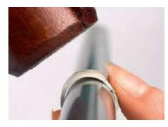
8. Form Perfectly Round Rings on Tapered Mandrels: When forming rings and bangles on tapered mandrels, keep turning the metal around the mandrel to counteract its tapered shape and to ensure that both edges become the same size.
