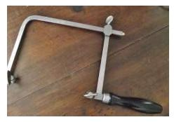
4. **Smooth Sawing from the Start:** Begin sawing with the blade tilted at a slight angle; then return to a vertical position to continue sawing sheet silver.
